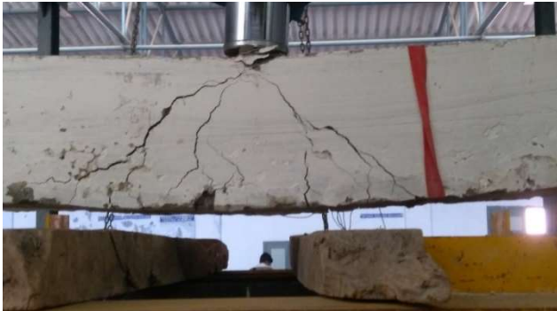
Fig.12. Comparison of flexural cracks- Analytical and Experimental
