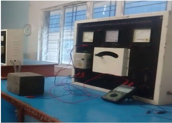
Figure 2: Electrical resistivity setup
